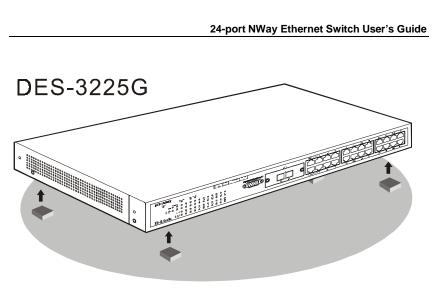
Figure 2-1. Installing rubber feet for desktop installation
